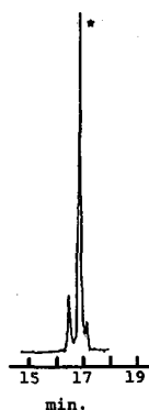
Fig. 3. Initial separation of cytochrome c mixture (85% BCc, 10% HCc and 5% DCc) by reversed-phase gradient elution. Conditions: column, 25 × 0.46 cm I.D. 5- \mu m DuPont Zorbax Bioseries Protein PLUS; 5–60% acetonitrile in water (plus TEA and TFA) gradient in 20 min; flow-rate, 1 ml/min; ambient temperature; 5 \mu g injected (small sample).
